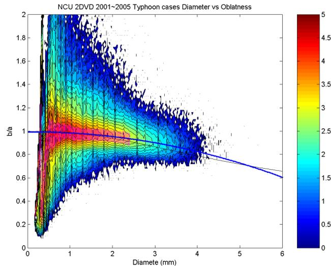
Fig. 2: (a)  $\log_{10} [N(D_e, b/a)]$ , where  $N(D_e, b/a)$  is the number of drops with each corresponding equivalent diameter  $D_e$  and axis ratio  $b/a$  in typhoon cases. The black solid line represents the DSR from Brandes et al. 2002 and the blue solid line represents the 2nd order fitting of DSR from typhoon systems. The pink bars represent the standard deviation of the average oblateness for each corresponding equivalent diameter.
