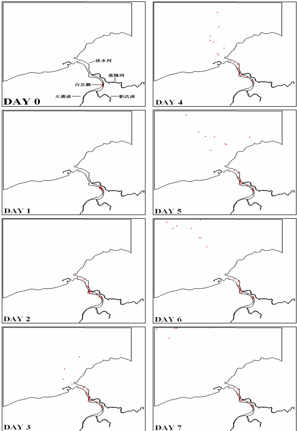
Figure 2. Model simulation of particles tracking: particles release from Taipei Bridge (Danshuei River) under mean flow conditions.
