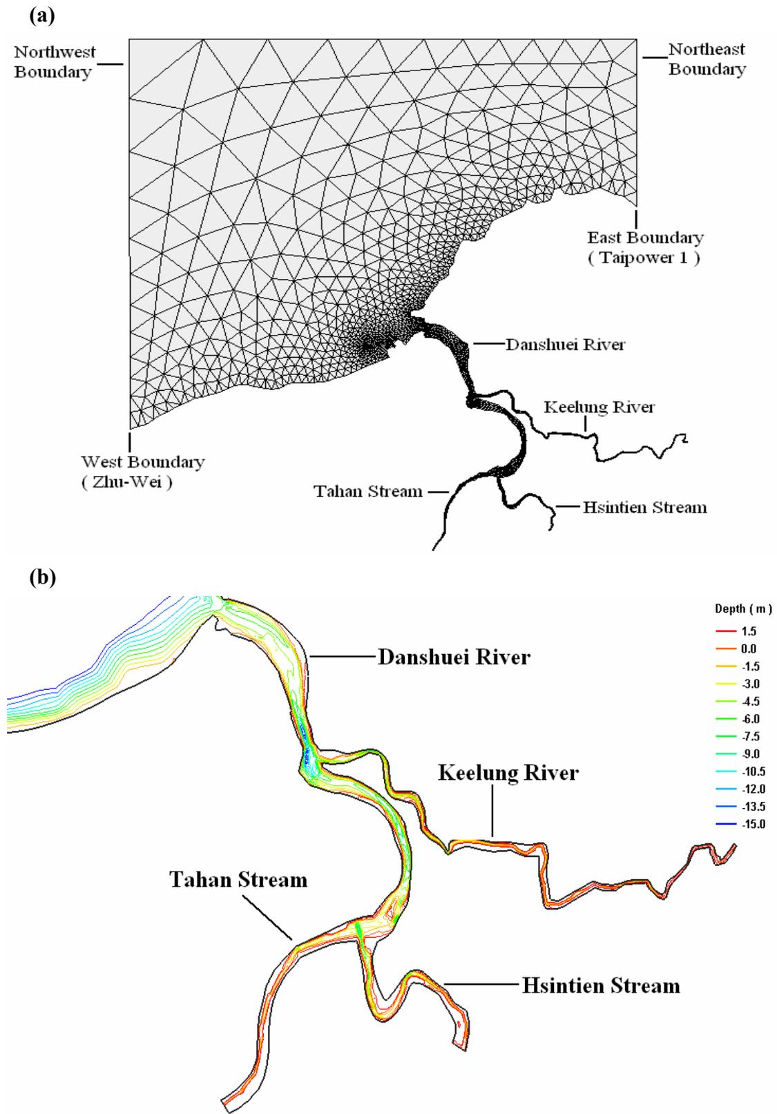
Figure 1. (a) An unstructured grid representing the modeling domain, (b) contour of bottom topography in the Danshuei River estuarine system.
