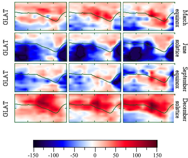
Figure 2. Field-aligned ion flow velocities observed by ROCSAT at 600 km altitude for geographic longitude versus geographic latitude in year 2000. The plots are arranged as in Figure 1. The ion flow parallel to the field line (northward) is shown in red color and anti-parallel to the field line (southward) in blue.
