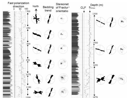
Fig. 4 Comparison of the fast-shear polarization direction with bedding trend determined from borehole images and fracture orientations measured from core images. Azimuths of the Chelungpu fault (CLF,  $20^\circ$ ) and maximum horizontal principal stress ( $S_{Hmax}$ ,  $115^\circ$ ) determined from earthquake focal mechanisms in central western Foothills of Taiwan are shown for references.
