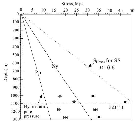
Fig. 2 Plot of overburden stress ( $S_v$ ) from integration of density logs, hydrostatic pore pressure, and  $S_{Hmax}$  (filled symbol) and  $S_{Hmin}$  values (open symbol) determined from leak-off tests at different depths. Dotted line shows the location of FZ1111. Heavy dashed line indicates the upper limit of the stress magnitude for a strike-slip fault stress regime with a coefficient of friction  $\mu=0.6$ .
