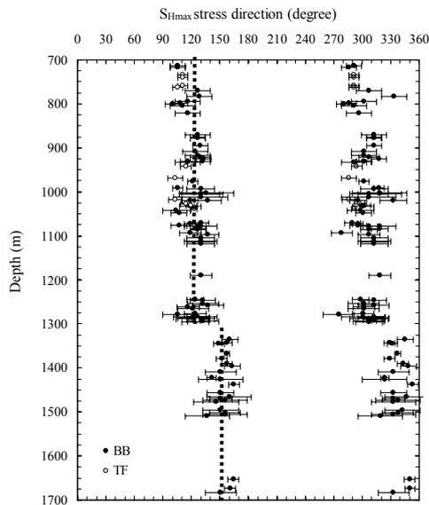
Fig. 3 The plot of azimuth of  $S_{Hmax}$  determined from breakouts (BO) and tensile fractures (TF) in the TCDP wells. Width of bar shows an opening angle of BO and TF with dark and open circles, respectively, as mid-point. Dotted lines are average of mid-points.
