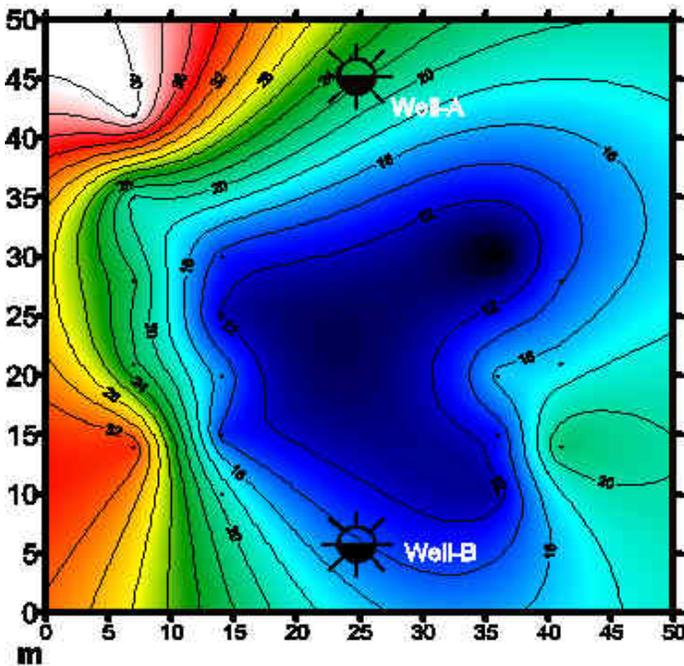
Fig. 1 The background apparent resistivity (in ohm-m) contour maps of frequencies (a) 128Hz (skin depth ~500 m) and (b) 4 Hz (skin depth ~1000 m), respectively, in TCDP area before water injection. Dots in each map indicate the sounding points. Note that low resistivity anomaly, indication of water, migrate to the SW at shallow depth ~500 m, while concentrate in between well A and B at depth ~1000 m. The repeat CSAMT survey
