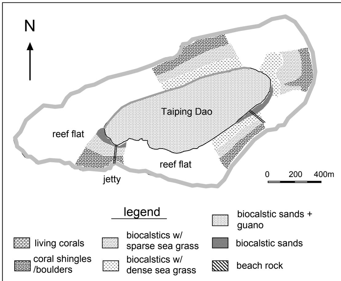
Figure 1. Sedimentary facies of the islet and reef flat of Taiping Dao, Nansha Islands.
