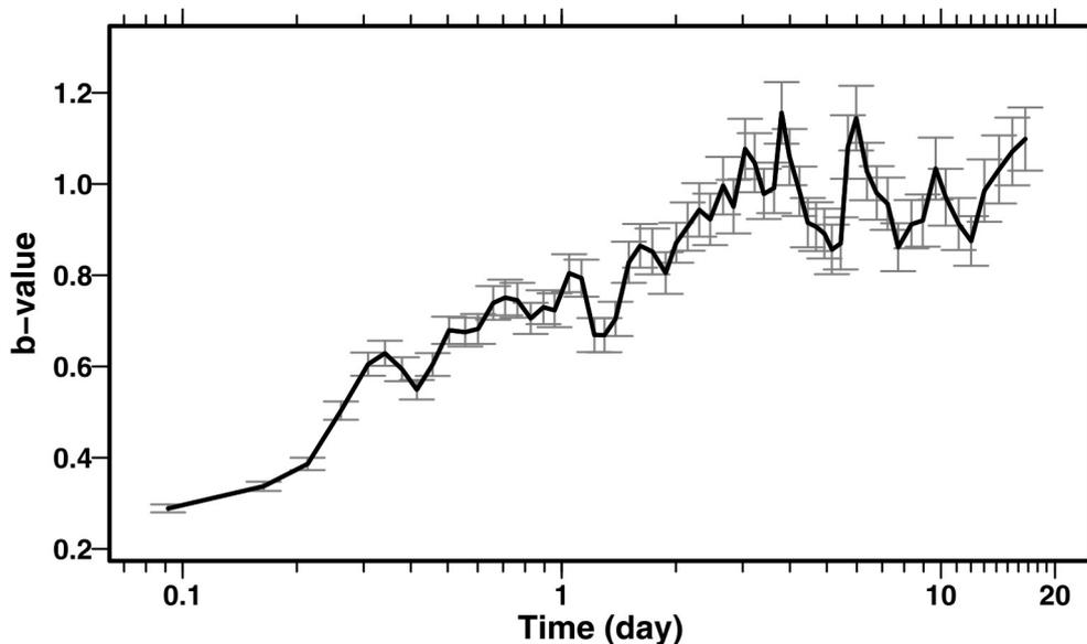
Figure 1. The time-varying b values for the aftershocks 12 hours after the Chi-Chi earthquake. The b values and the associated standard errors are computed based on a moving time-window containing 250  $M \geq 2.5$  aftershocks sliding by 100.
