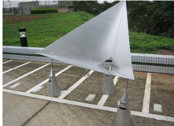
Figure 1. Trihedral corner reflector with 1.6 meter sides, whose response to an incident signal is returned in its direction (a feature making them treatable as point targets).
