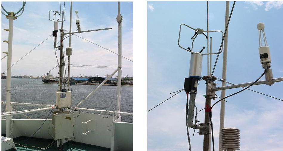
Figure 2. (left) Eddy covariance system installed in OR1 during the OR1-802 cruise at the Kaoshiung Harbor on 18 July 2006. The flux was measured at 12.12 m above the ocean surface. The two boxes in the lower mast were the control box of infrared hygrometer and Dateallogger (CR5000); (right) Three-axis sonic anemometer (Young 81000) and infrared hygrometer (LICOR 7500) used to measure the fluxes.
